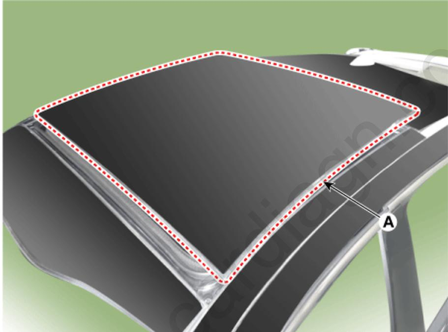
2. Remove the both sides mechanism cover (A).
